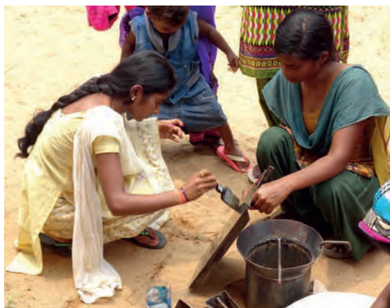
Young Women preparing the metal mould to make the Fuel Efficient Stoves
